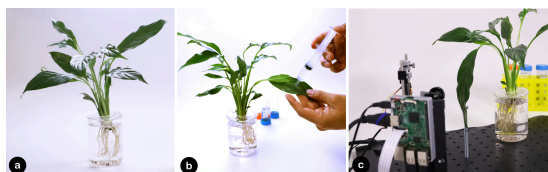
Fig 7. a) Spathiphyllum plant in DI Water culture, b) Leaf infusion of oligo-functionalized CNTs through the abaxial side of the leaf. c) Laser diode to excite the dsDNA nanosensors inside the leaf. While fluorescence and subsequent quenching is observable in the visible domain, RPi digital detection can bridge plant detection to digital software and aid in long term observation/logging.
