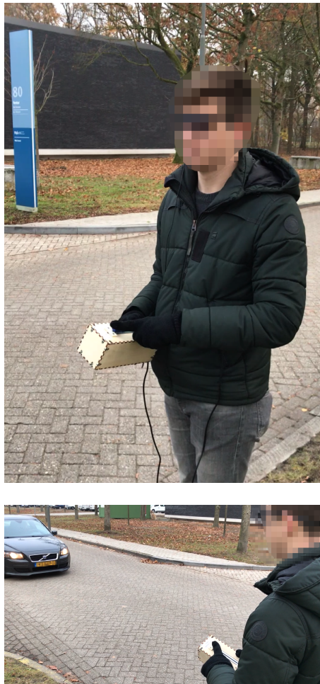
Figure 2: Experiment setup - the pedestrian stands on the pavement at the edge of the road with the input device in his hands, and manipulates the slider in real time as the vehicle approaches
