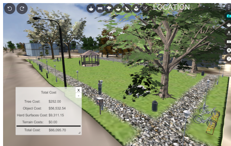
Figure 2: Land.Info provides estimated costs and several environmental parameter impacts based on applied design
