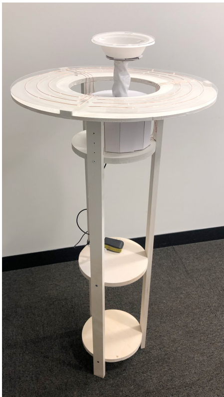
Figure 1: Prototype of SociaBowl, a table with an actuated bowl as a centerpiece to help mediate group conversations.
