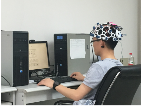
Figure 5: The experiment and OpenBCI device. We adapt OpenBCI Cyton board with the 3D printed headset to acquire raw EEG signals and the data are delivered to the computer via Bluetooth. The neuro-headset feature 8 channels (Fp1, Fp2, C3, C4, T5, T6, O1 and O2) plus 2 references (A1 and A2) based on the 10-20 format. The sampling rate is 250. We develop the trigger function and hardware parts to help segment the data precisely.
