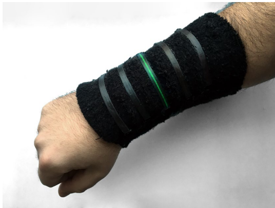
Figure 1: Howel, representing 3rd intensity zone via the green line on the 3rd stripe.
