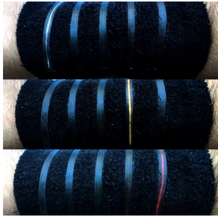
Figure 3: Examples for HR zone representations on the Howel: (Top) 1 st HR Zone; (Middle) 4 th HR Zone, (Bottom) 5 th HR Zone.
