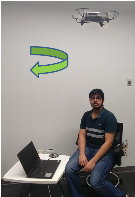
Figure 5: Rotating the chair to rotate the drone
