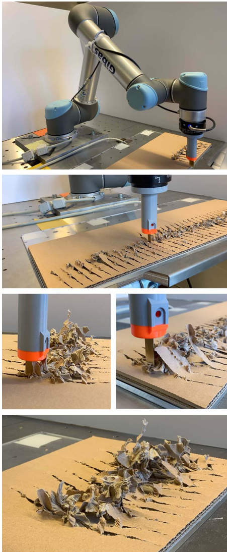
Figure 4: An emergent material effect was discovered: the cardboard material ripped and accumulated in parallel to the cutting operation. The extruded material is eventually pulled out of the cardboard surface by the lift of the end-effector.
