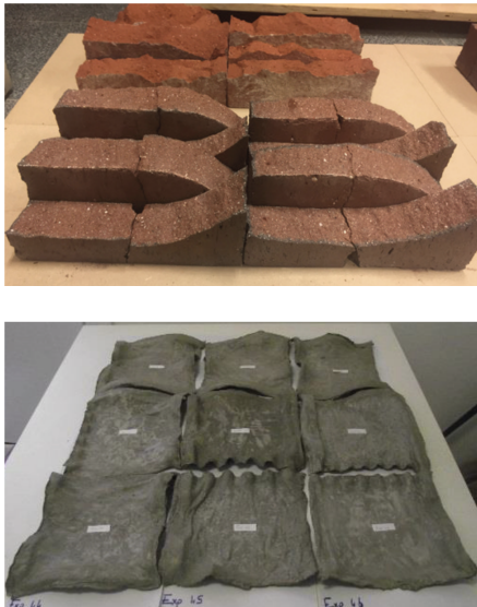
Figure 2: A few examples of our exploratory experiments on the digital fabrication of emergent material effects on different building materials. Top: bricks that were purposefully broken along curved surfaces, revealing more natural stone surface textures. Bottom: robotically folded and squished fibre cement panels after drying, revealing handmade-like topographies.
