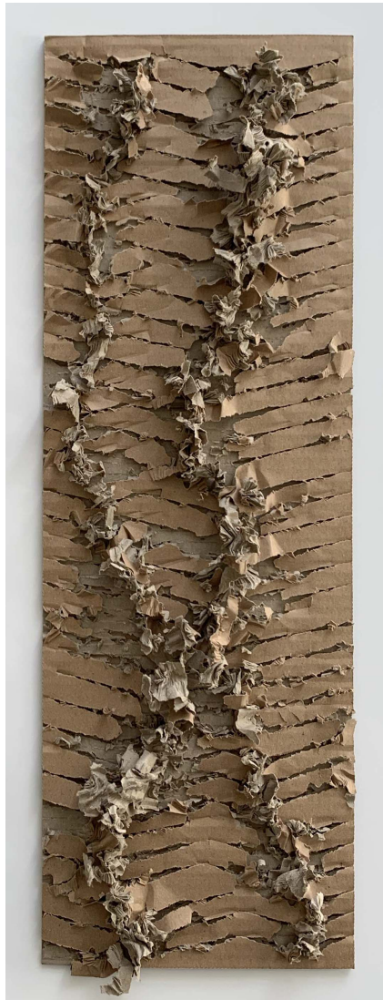
Figure 1: Designing 'with' fabrication operations: an example of reproducing variations of an emergent material effect on corrugated cardboard via cutting operations.
