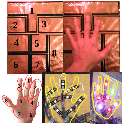
Figure 5: The first BalBoa prototype measures 8 key pressure points in the hand (upper left image). The device is reset when turned on, and from there, the pressure values are read every 50ms. A hand display, composed by 8 RGB LEDs (bottom-middle and right image) is mapped to the corresponding pressure points. The individual LEDs' colors are updated within percentages of applied pressure (see Figure below). The bottom-right image shows the pressure distribution of a hand, with maximum pressure applied to the middle finger (n°1), upper palm (n°4,5) and a point in the lower palm (n°7); and the less pressure in the thumb (n°8).
