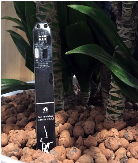
Figure 5: The sensor stick detects moist, light and temperature.
