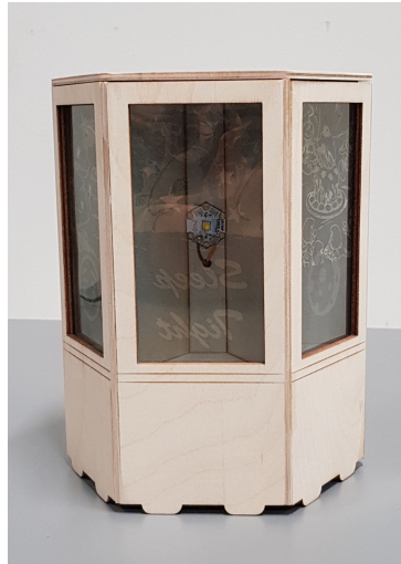
Figure 3: ShadowLamp design with electrochromic displays.
