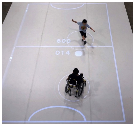
Figure 1: Two children competing on iGYM's interactive floor. The projected circles around their bodies can be expanded – through body movement or with a push button – to manipulate a virtual target on the floor.
