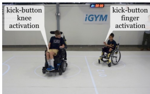
Figure 4: Two examples of push button activation; knee (left player) and index finger (right player).
