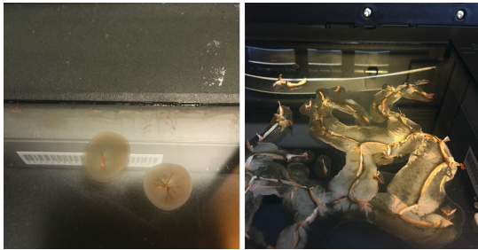
Figure 6: Dried, dead layer of mold cells. Left: small patches of Moldy Ghosts. Right: A larger structure of Moldy Ghosts, covering a top right hand corner of the scanning bed. These layers of mold were adhered onto the glass surface of the scanning bed, likely to have been caused by mold overgrowth.
