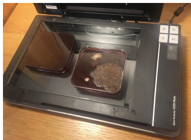
Figure 2: Flatbed photo scanner with two culture dishes, one upside down and one upright showing mold growth. When the dish is upside down (during imaging), a 3mm gap is present between the surface of the scanning bed and the culture dish, allowing space for mold to grow. This microbe imaging technique was introduced by van Eck and Lamers [22].
