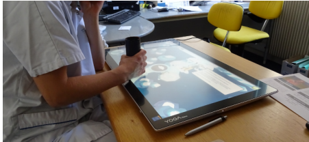
Figure 1: Ergotact is composed of a serious game on a table top. The therapist holds a tangible object covered with force sensors distributed around the surface. This tangible object is used to interact with the game deployed on the tabletop.
