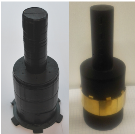
Figure 2: Left : One of the prototype featuring 63 mm (Bottom part) and 28 mm (top part) handle diameters, Right : Object prototype revealing one unit of force sensors. Weight : 250 g
