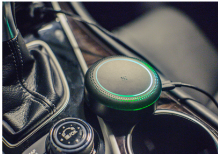
Figure 3: Voice-reactive microphone while in speech detection mode.
