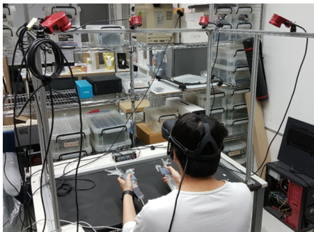
Figure 4: The experiment environment for Experiments 1 and 2. An optical tracking system was used to track the controllers and the thumbs.
