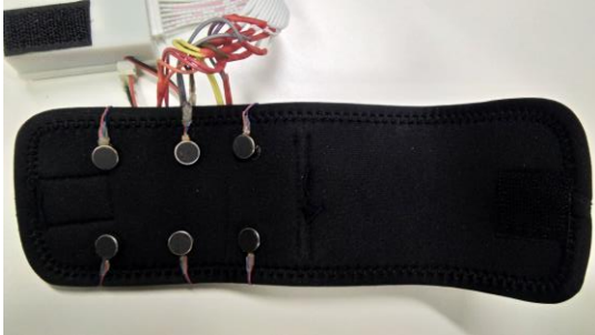
Figure 2: Flat type vibration motors attached on a sport wristband.
