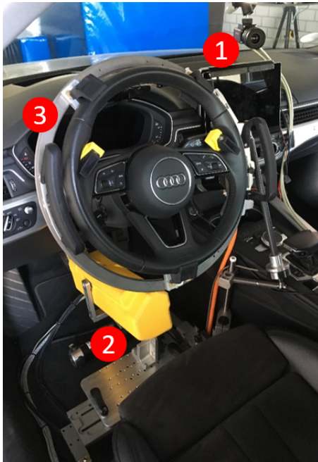
Figure 3: Test vehicle setup: tablet (1) for self-ratings with KSS; driving robot on pedals (2) and steering wheel (3)
