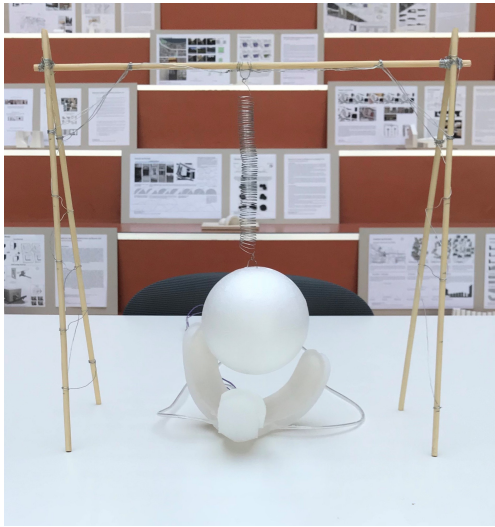
Figure 1: The setup of the Helpless Soft Robot: The robot trying to grab the ball using the “Grabbing” motion where all three parts of the actuator are inflated lightly.
