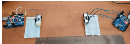
Figure 2: Testing the code transmission between the ultrasonic sensors.
