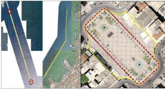
Figure 3: Scenario 1 (left) involved measuring the distance between the first and the fourth pillar of a well-known bridge and the breakwater's length in the old harbor. Scenario 2 (right) involved measuring the inner area of a popular square located in the city's center (red dotted-line rectangle) and modifying this area to include the side parts of the square (yellow solid-line polygon).
