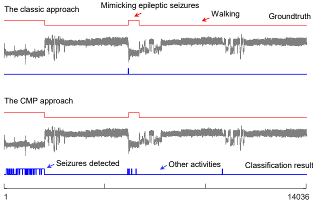
Figure 22: Classification result with the dictionary learned using classic motif search (top) and the dictionary built using the guided motif search approach (bottom).
