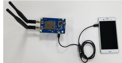
Figure 1: DSRC V2P prototype module attached to smartphone via USB port
