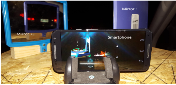
Figure 7: CamMirror setup for vehicle ranging
