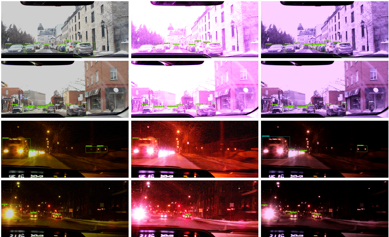
Fig. 12. Qualitative object detection results. While the images produced by an ISP with expert-tuned parameters (left) may look more natural to the human eye, the performance of a pretrained object detector can be improved by adjusting the ISP parameters to maximize the intersection-over-union score (IoU) of the detector (right). The middle column shows the detection results with the initial tuning parameters.
