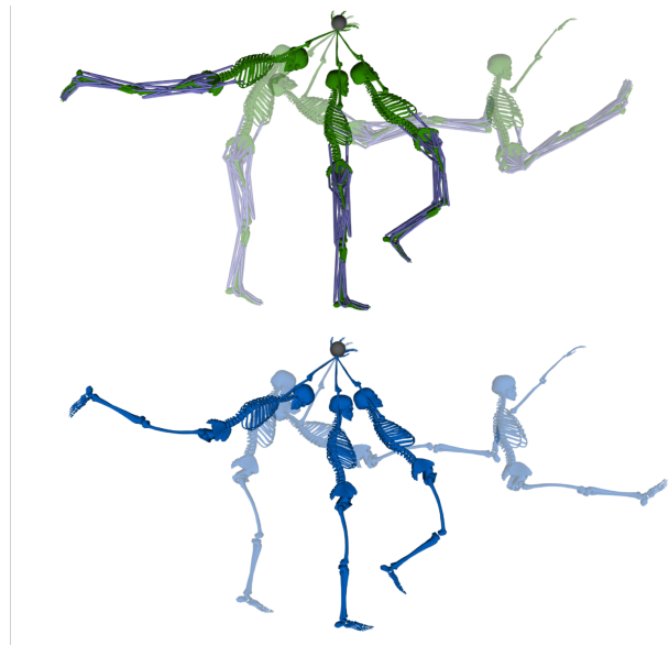
Fig. 1. Top: A swing motion solved by trajectory optimization in the muscle-actuation space. Bottom: Our proposed method can solve the same task in the joint-actuation space, yielding similar motion but costing fewer iterations and less computation time.
