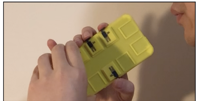
Fig. 14. Saxophone app. We demonstrate a 4-key “smartphone's saxophone”. Each Vidgits button serves as a saxophone key. By detecting the downstroke and upstroke of each Vidgits button, this smartphone application can recognize which keys (and key combinations) are pressed and play the corresponding music notes.
