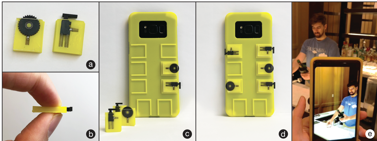
Fig. 1. Vidgits widgets. We design a family of physical widgets that are modular, power efficient, (a) compact, and (b) thin. (c) These widgets can be attached to a smartphone's protective case in a modular fashion. (d) The widgets can be used to construct a wide range of user interfaces and adapt to individual's preferences. (e) As just one example, here we use a Vidgits knob to zoom a camera's field of view and a Vidgits button to trigger the capture. In this way, the user can easily take a photo with a desired focus using a single hand, without needing another hand to pinch on the screen. We demonstrate several more applications in the paper.
