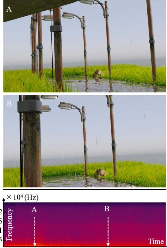
Fig. 1. Audiovisual simulation of walking along a country road in the rain. Frames A and B illustrate two positions of the listener. From A to B, as the listener gets closer to the street lights, the metal sound effects become more and more apparent. Our method is able to capture this dynamic change of rain sound as shown in the spectrogram on the bottom row.
