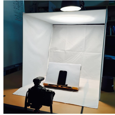
Figure 19: To take a picture needed for smug attack, a smart-phone was placed under a bright light source, and in front of a high-resolution camera.
