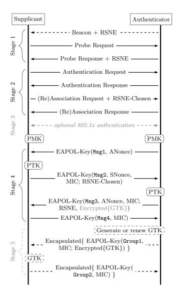
Figure 1: Frames sent in the 802.11 handshake, including their most important parameters. Optional stages or parameters are shown in (dashed) gray.
