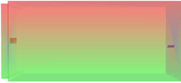
Figure 7: SfePy simulation output for a non-defective tetrahedral prism, reconstructed using our methodology (Fig. 4). As expected, the simulation does not show any abnormal stress points.
