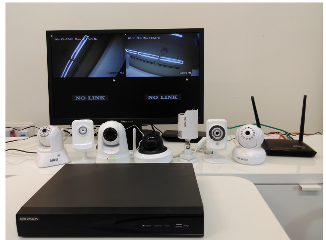
Figure 5: Setup of Cameras and NVR in Lab.
