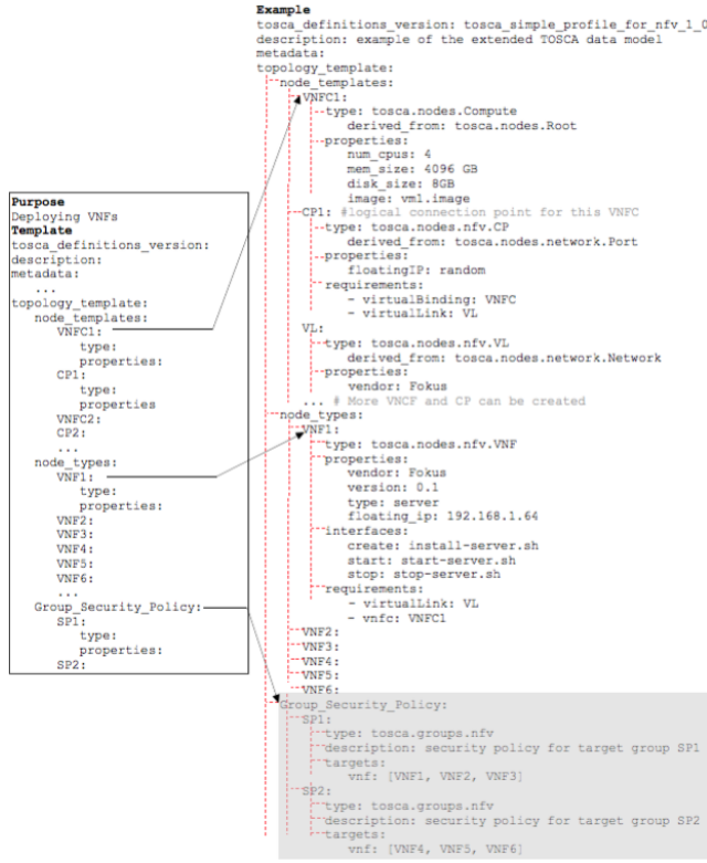
Figure 4: The extended TOSCA data model with security policy specification (highlighted in grey)
