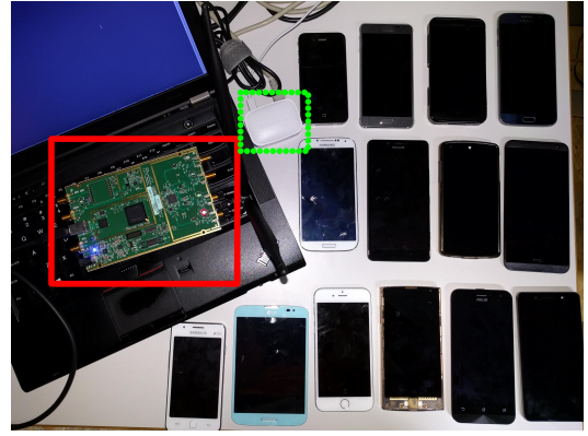
Figure 1: Our experimental setup, showing the USRP (left), a Wi-Fi access point (center, dotted square), and our test phones.
