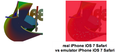
Figure 5: Visualization of the rendering differences between an emulated and real iOS device using the same software stack. We indicate in red the per-pixel Picasso solution differences.
