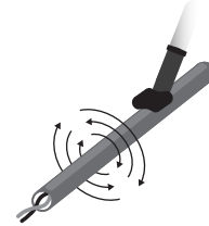
Figure 5: Near Field/H-Probe used to capture the radiated electromagnetic fields around an Ethernet cable.
