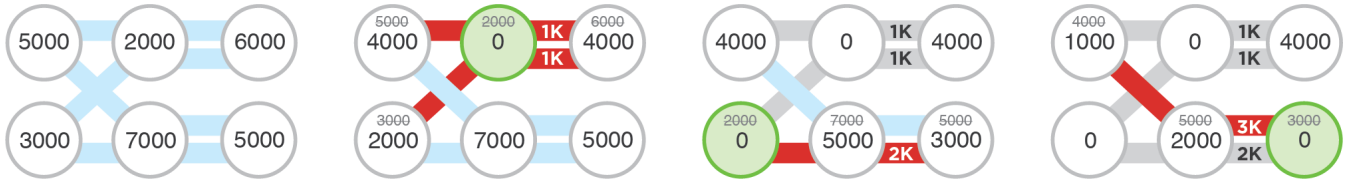
Figure 1: Example of circuit bandwidth estimate algorithm. Each step the relay with the lowest bandwidth is selected, its bandwidth evenly distributed among any remaining circuit, with each relay on that circuit having their bandwidth decremented by the circuit bandwidth.
