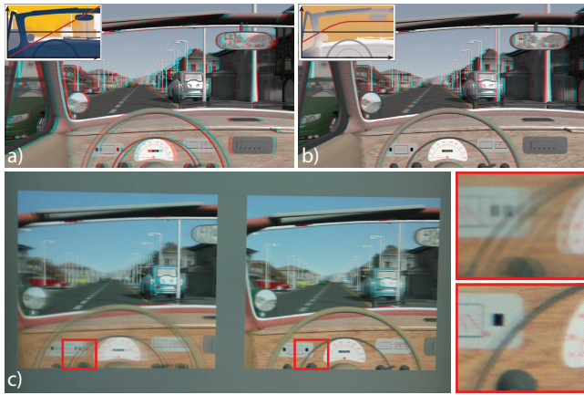
Figure 8: Example of disparity compression for autostereoscopic displays. a) The original linear compression with the corresponding disparity map and mapping curve shown in the inset. b) Our manipulation applied on top of (a) to compress stronger regions that benefit from motion parallax. c) A photo of our display. Aliasing artifacts are pronounced in the content with only linear mapping (insets).
