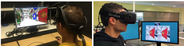
Figure 7: Our user study Setups. Left shows our desktop setup with a high-speed gaze tracker, and right is our HMD setup with a gaze-tracker integrated within the HMD.
