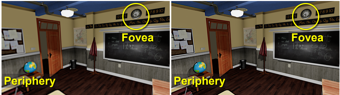
Figure 1: Our classroom scene with eye fixation at the yellow reticle. (Left) Our perceptually-validated target foveated image. (Right) Our proposed foveated rendering system that avoids shading up to 70% of the pixels and closely matches the frequency content of our target by using pre-filtered shading terms, contrast preservation, and applying a new temporal antialiasing that improves temporal stability by an order of magnitude (providing stability similar to a temporally antialiased non-foveated renderer).
