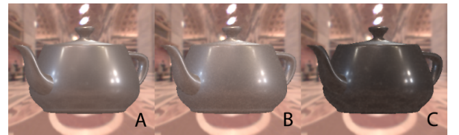
Figure 13: Our functionals allow to define similarity metrics based on individual appearance attributes. While A-B and A-C are very similar according to RMSE, A-B exhibit a much lower distance in terms of brightness than A-C.
