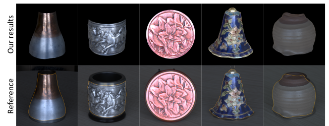
Figure 7: Qualitative Validation. Side-by-side comparisons of reference photographs and recovered shape and surface reflectance visualized under a novel lighting conditions different from the acquisition environment.
