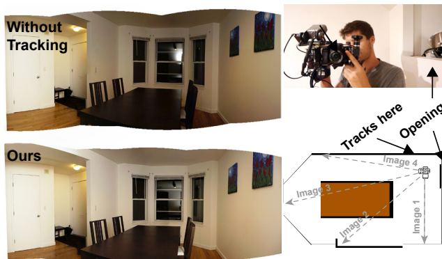
Figure 14: Handheld Panorama with Surface Tracking: Without tracking (above), the virtual light starts out on a good bounce surface, but begins to point through an opening in the wall as the user rotates their camera to capture more images. Notice that the table is underexposed, and a harsh reflection of the bounce flash can be seen in the window. By using our system to track camera movement and keep the flash pointed at the initial bounce surface (below), we achieve better and more consistent lighting across all input images.
