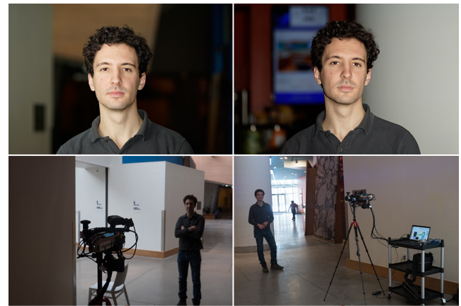
Figure 5: Direct flash produces harsh illumination. Static flash directions work in some configurations, but do not adjust to subject pose, surface reflectance, or scene geometry. Our prototype takes these factors into account, which leads to consistently good illumination.
