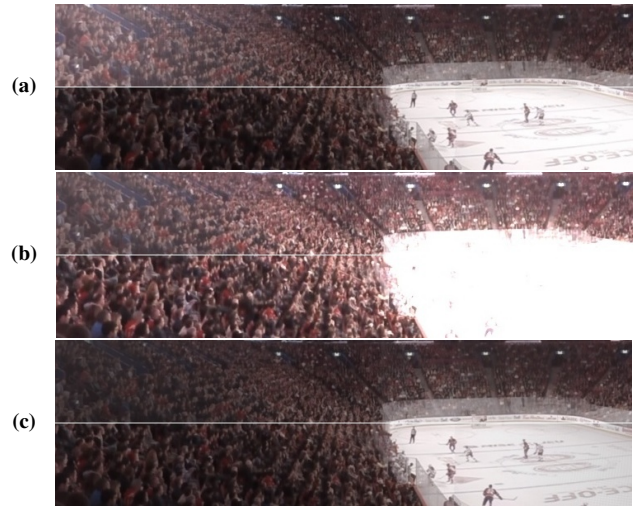
Figure 13: A scene containing significant exposure variation, with the top half of each image cropped from the left eye's panorama and the bottom half cropped from the right eye's. (a) No exposure correction - the left edge of the image is hard to fuse due to exposure differences. (b) Exposure correction applied and resulting HDR image clamped to 8 bits - the rink is blown out. (c) Exposure correction followed by tone mapping to match input exposures.
