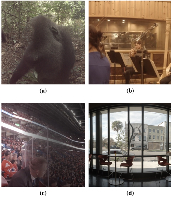
Figure 17: Failure cases - crops from one eye of the ODS stitches. (a) As objects get closer than the limits described in section 4.3 stitching completely breaks down, here the gorilla is ~15cm from the camera. (b) Thin structures can be missed in the flow computation stage which leads to ghosting on the mic stand and bow. (c) Semi-transparent surfaces can deform as shown here. (d) In very rare cases flow mismatches occur. Here a combination of the correct match being occluded and repeated texture providing a good match in the wrong location leads to a severe warp.
