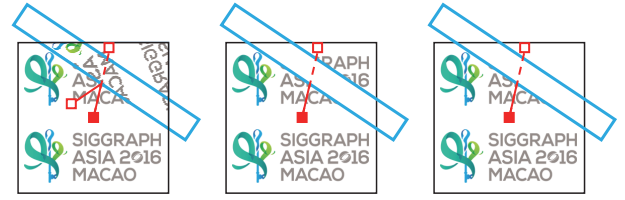
Figure 7: Schematic depiction of three strategies to evaluate the modified height field \bar{h} within the shadowed convolution (17), in an example where a blue obstacle intersects with the kernel window. The red pixel is the center of the kernel, where the acceleration is computed. The white pixel is one particular pixel that contributes to the convolution. From left to right: (i) reflection of height values about the obstacle normal (accurate but costly); (ii) zeroing of height values within the obstacle (cheap but inaccurate); (iii) zeroing of height values within obstacle shadows (our proposed compromise).
