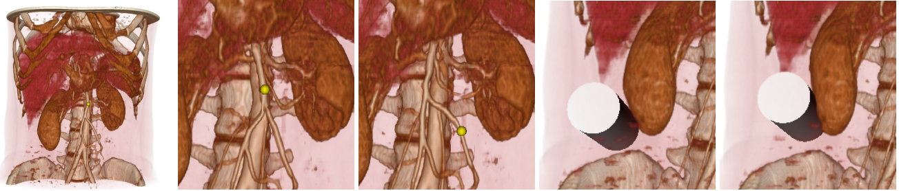
Figure 1: Interactive deformation of a CT data set discretized with 281K tetrahedra. With our corotational coarsening method, we represent this complex model using a coarse mesh with 6K tetrahedra, which captures the high-resolution heterogeneity of the original model. As shown in the examples, we can impose accurate boundary conditions at arbitrary locations within the volume (see the yellow ball pulling from the veins, or the cylindrical tool in contact with the kidney).
