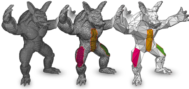
Figure 5: The three decimation levels of a mesh. The input mesh (left) has 346k faces, the redundancy free mesh (center) has 29k faces and the minimally sampled mesh (right) has 1000 vertices. Note how the guiding regions defined in the redundancy free mesh are preserved in the minimally sampled mesh.
