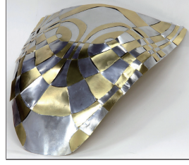
Figure 22: Woven principal strips for sheet metals. Hood of the automobile is fabricated by sheet metals of principal strips.
