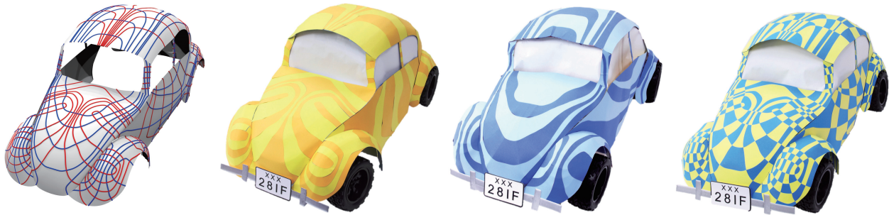
Figure 1: Left to right : Computation of orthogonal net of lines of curvature of automobile surfaces. Two-layered principal strips (maximum principal strips on the visible side). Two-layered principal strips (minimum principal strips on the visible side). Woven principal strips.
