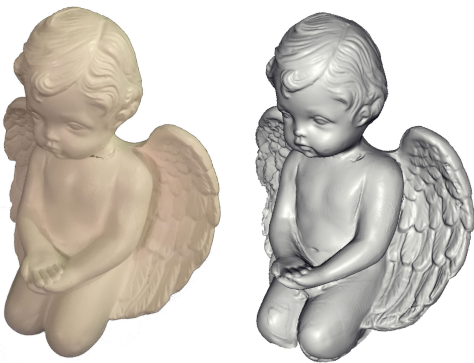
Figure 13: A 20 cm tall angel figurine (left) is scanned and reconstructed (right) using our system, with the object platform adjusted to three heights.
