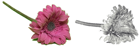
Figure 15: A flower with a long, thin stem (left) is scanned and reconstructed (right) with our system. Elongated objects such as this are a worst case for a turntable-based system with equally-spaced views.
