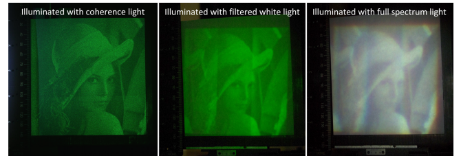
Fig. 12. Results of an offset pairing example illuminated by a coherence green light source (left), broadband green light source (center) and a full spectrum white light source (right). (Lena Photograph by Dwight Hooker)
