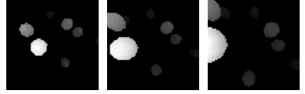
Fig. 5. The synthetic vision images (64x64 pixels) from the viewpoint of the dragon in flight. The depth images were taken from the z-buffer of the OpenGL rendering pipeline.
